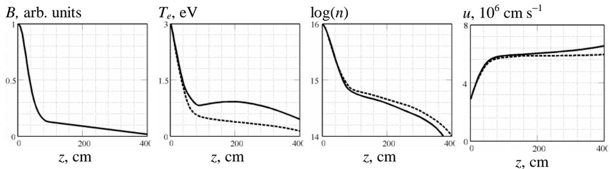
Fig.3. Longitudinal distributions of magnetic field  $B$ , temperature  $T$ , density  $n$ , and flow velocity  $u$  and supersonic plasma jet in the magnetic nozzle ignoring recombination (dotted line), subject to recombination (full line). Boundary conditions in the throat ( $z = 0$ ):
