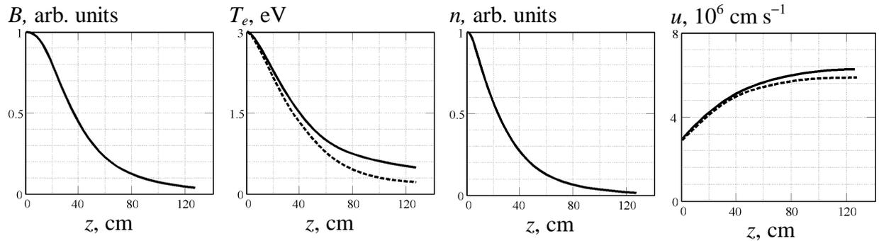
Fig.1. Longitudinal distributions of magnetic field  $B$ , temperature  $T$ , density  $n$ , and flow velocity  $u$  and supersonic plasma jet in the magnetic nozzle ignoring recombination (dotted line), subject to recombination (full line). Boundary conditions in the throat ( $z = 0$ ):
