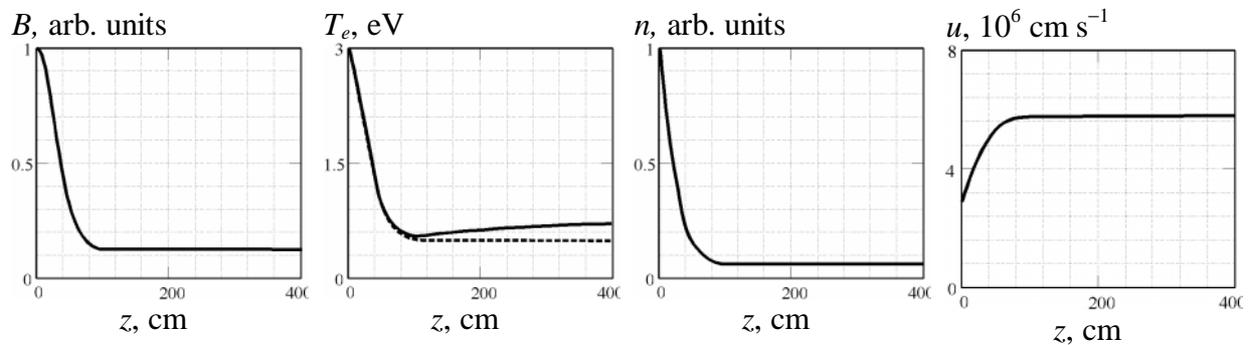
Fig.2. Longitudinal distributions of magnetic field  $B$ , temperature  $T$ , density  $n$ , and flow velocity  $u$  and supersonic plasma jet in the magnetic nozzle ignoring recombination (dotted line), subject to recombination (full line). Boundary conditions in the throat ( $z = 0$ ):
