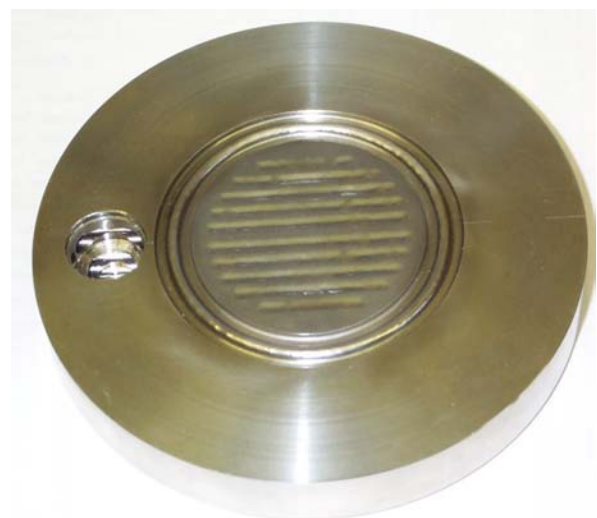
Figure 4: Beam absorber, view from proton beam side.
