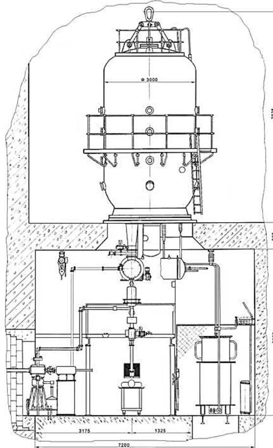
*Fig.3 Layout of the accelerator under running with unseparated beam focused at the beryllium target.*
