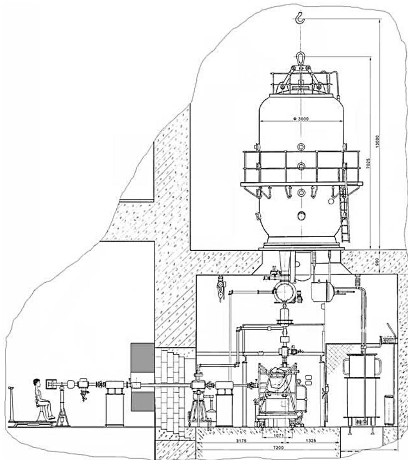
*Fig.4 Layout of the accelerator under running with the separated beam in the horizontal part of the beam line and the lithium target installed.*
