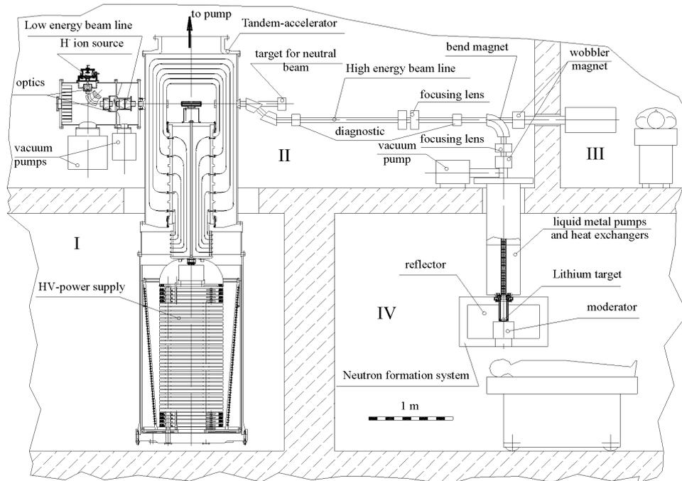
*Fig. 1. Possible variant of neutron source.*
