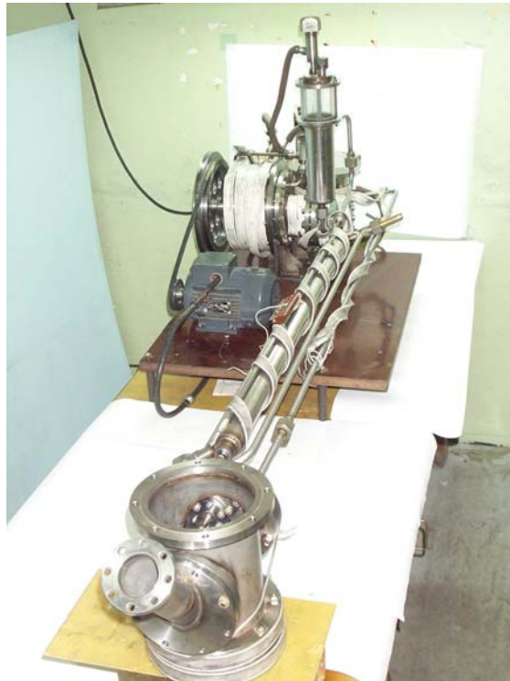
Fig. 2. Liquid metal cooling system.
