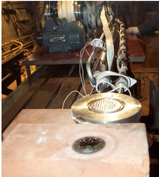
Fig. 3. Target before irradiation by electron beam.
