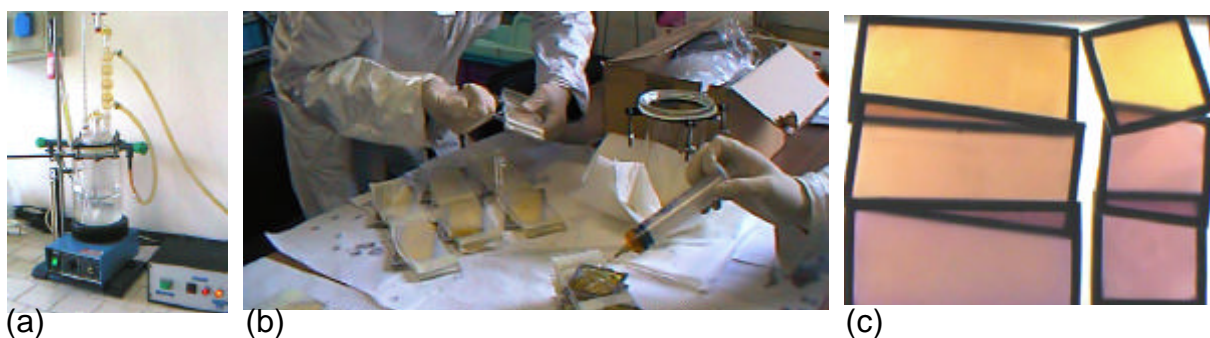
Fig. 3 – The apparatus for gel dosimeter preparation (a), the final operation of performing gel samples (b) and some dosimeters irradiated at different \alpha -doses (c).
