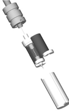
Fig.1. Artistic view of the avalanche confinement TEPC with replaceable cathode walls.
