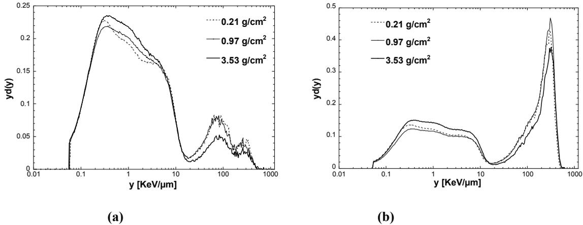
**Figure 2.** (a) Without  $^{10}\text{B}$  microdosimetric spectra at different polyethylene depths; (b) With 100 ppm  $^{10}\text{B}$  microdosimetric spectra at different polyethylene depths.
