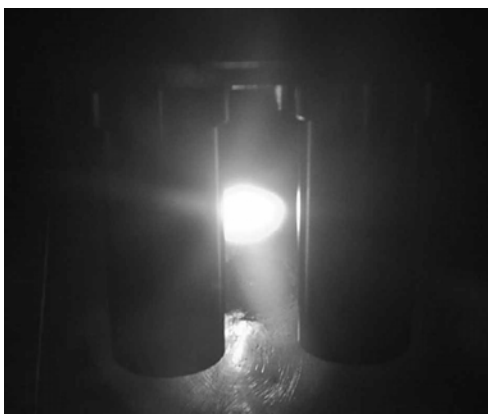
Fig.3. Thermal spot, produced at Faraday cup plate by 7 mA, 20 KeV H^- beam
