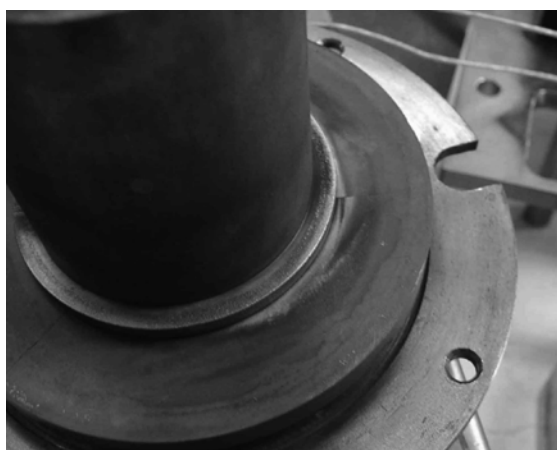
Fig.5. Metal deposited to cathode-anode insulator
