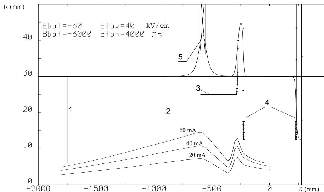
Fig. 2. Envelope of the 12 keV, 60 mA proton beam. 1, 2 – limiting diaphragms; 3 – beam pipe and vacuum tank; 4 – high-voltage electrode; 5 – magnetic lens.
