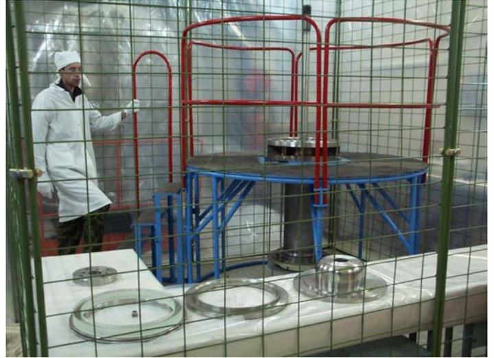
*Fig. 9. View of a tool for assembly of the tandem feedthrough insulator and "clean" room.*
