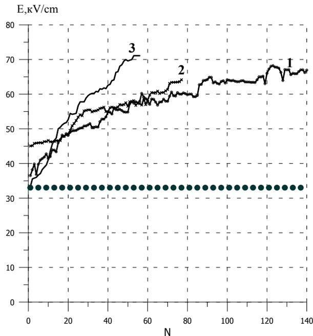
Fig. 4. Example of 3 training curves of 45 mm vacuum gap. 1,2 – 9 J; 3-31 J.
