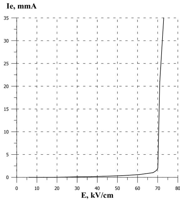
*Fig. 5. Full electrons emission current opposite electrostatic field intensity.*
