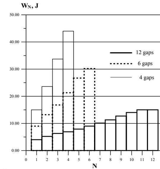
Fig. 2. Gap storage energy at high voltage electrode potential equal 1.25 MV.
