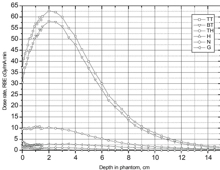
Fig. 8. Absorbed doses rates as function of depth in phantom.  $MgF_2$  moderator, size  $40 \times 40 \times 40 \text{ cm}$ , proton energy 2.3 MeV, beam current 1 mA. TT – tumor total dose, BT – boron dose in tumor, HT – total dose in healthy tissue, H – proton recoil dose, N – dose from nuclear reaction with nitrogen, G – gamma ray dose.
