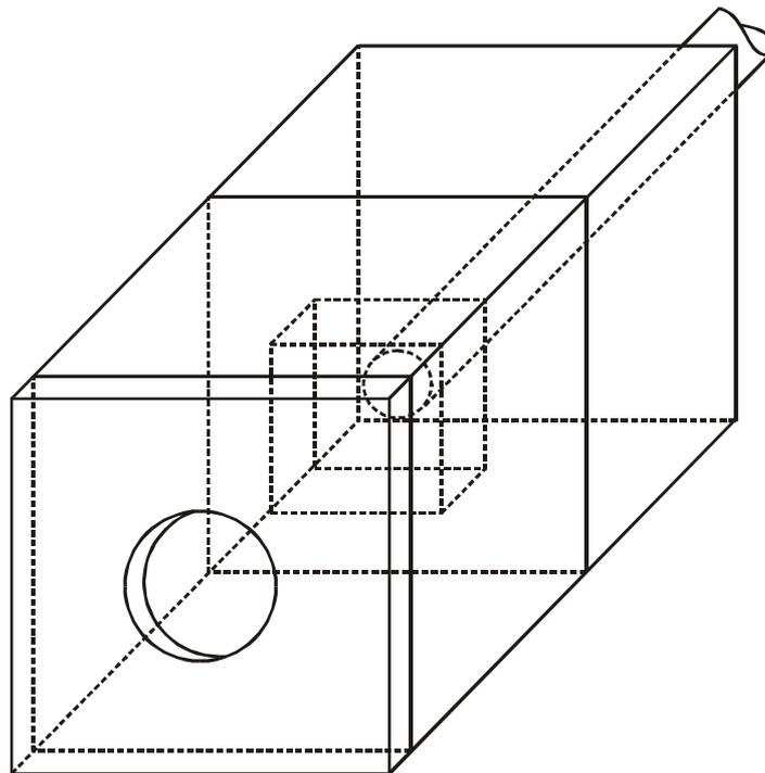
Fig 2. Beam shaping assembly calculation model for in-phantom absorbed dose distribution modeling.
