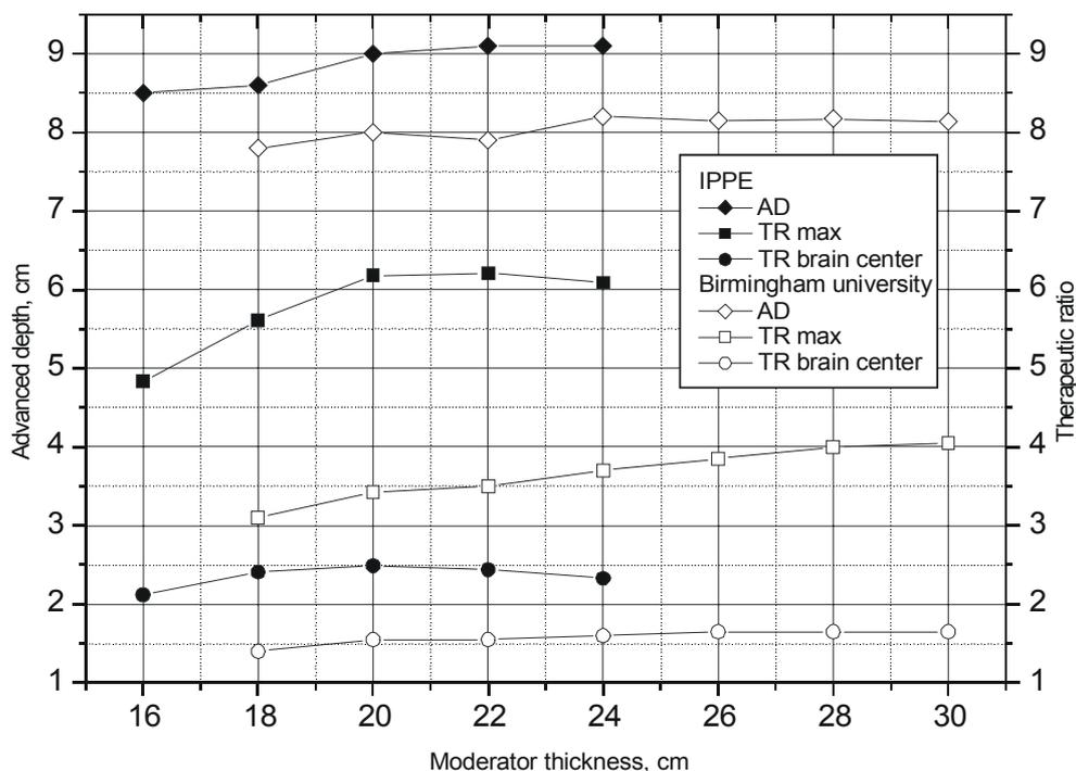
Fig. 13. Moderators characteristics comparison for MgF<sub>2</sub> – polytetrafluoroethylene moderator (proton energy 2.3 MeV) and moderator suggested by Birmingham University team [12] (proton energy 2.4 MeV).
