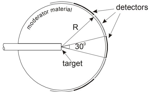
Fig. 1 Calculation model for evaluation in-air epithermal neutrons source characteristics.
