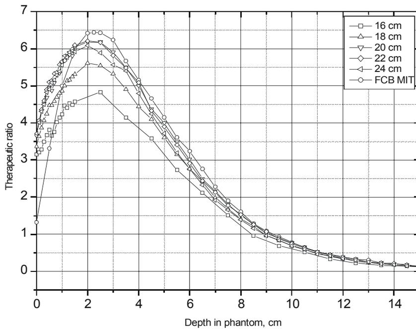
Fig. 12. Therapeutic ratio for MgF<sub>2</sub> – polytetrafluoroethylene moderator (size 40x40x40 cm) with various MgF<sub>2</sub> block length. Proton energy 2.3 MeV. FCB MIT – reactor based beam [13].
