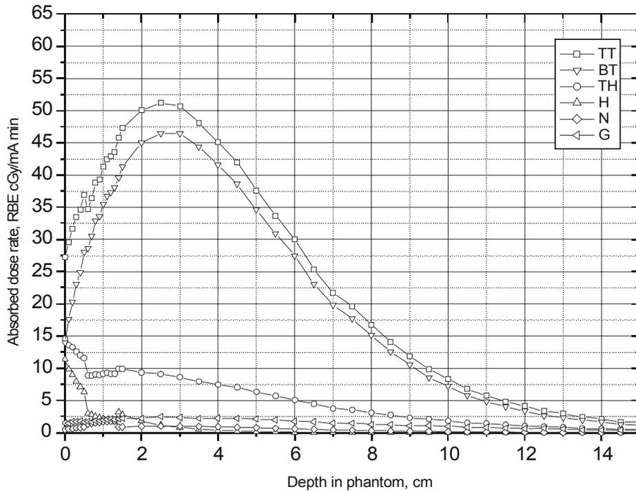
Fig. 10. Absorbed doses rates as function of depth in phantom. Fluential moderator, size 40x40x40 cm, proton energy 2.3 MeV, beam current 1 mA. TT – tumor total dose, BT – boron dose in tumor, HT – total dose in healthy tissue, H – proton recoil dose, N – dose from nuclear reaction with nitrogen, G – gamma ray dose.
