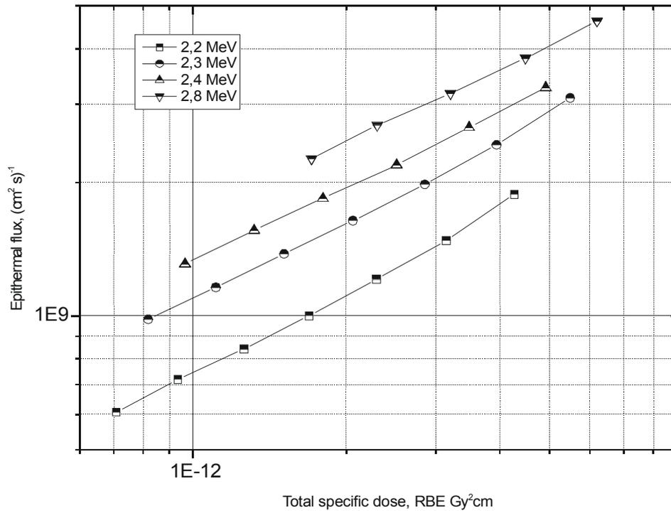
Fig 7. Epithermal neutron flux & total specific dose for MgF<sub>2</sub> moderator, various moderator sizes, collinear geometry. Moderator radius from left to right 28, 26, 24, 22, 20, 18, 16 cm. Thick lithium-7 target, proton energy 2.2, 2.3, 2.4, 2.8 MeV, proton current 10 mA.
