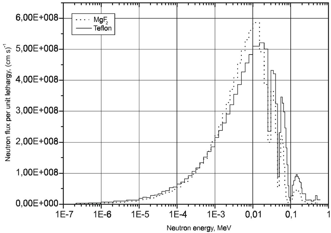
Fig. 5. Neutron spectra from MgF<sub>2</sub> and Teflon moderators with radius 20 cm on a proton beam direction. Proton energy 2.3 MeV, current 10 mA.
