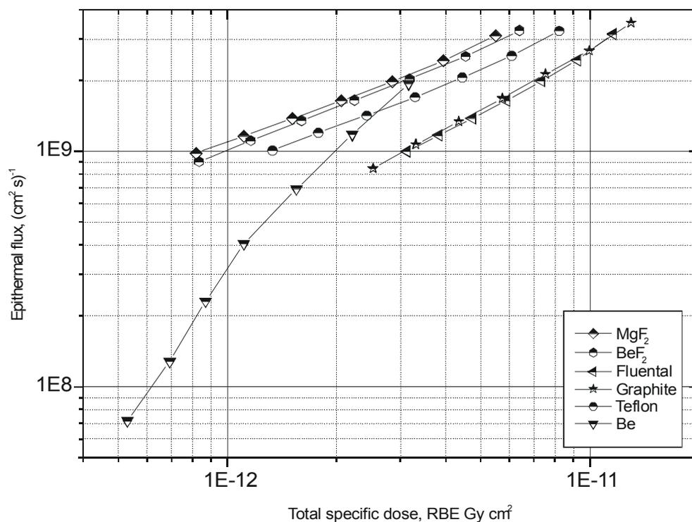
Fig 4. Epithermal neutron flux & total specific dose for various materials and moderator sizes for collinear geometry. Moderator radius from left to right 28, 26, 24, 22, 20, 18, 16 cm. For thick lithium-7 target, proton energy 2.3 MeV, proton current 10 mA.
