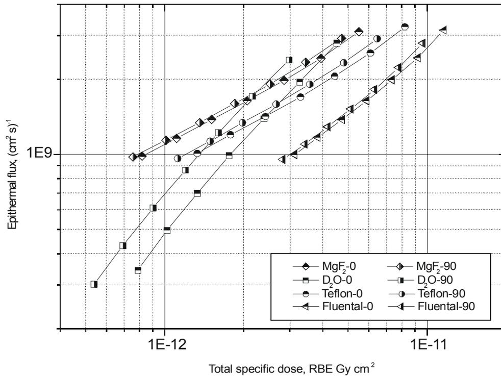
Fig 3. Epithermal neutron flux & total specific dose for various materials and moderator sizes for collinear and orthogonal geometry. Moderator radius from left to right 28, 26, 24, 22, 20, 18, 16 cm. For thick lithium-7 target, proton energy 2.3 MeV, proton current 10 mA.
