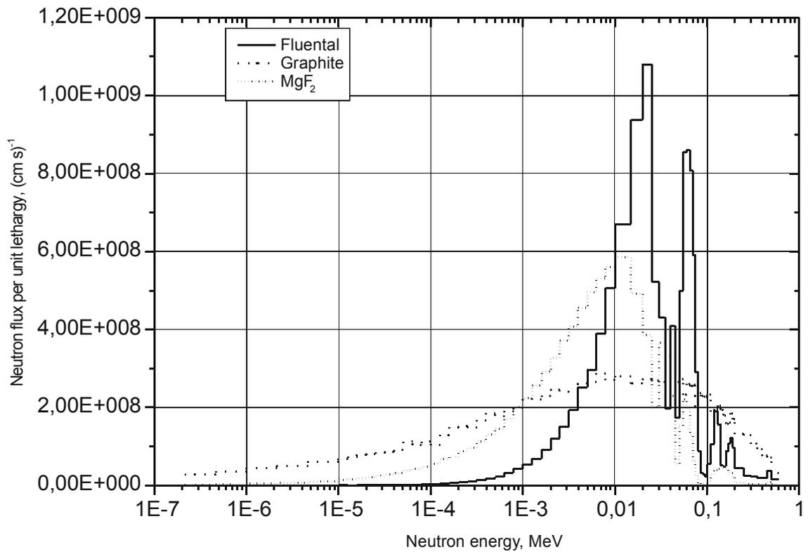
Fig. 6. Neutron spectra from Flualtal, Graphite and MgF<sub>2</sub> moderators with radius 20 cm on a proton beam direction. Proton energy 2.3 MeV, current 10 mA.
