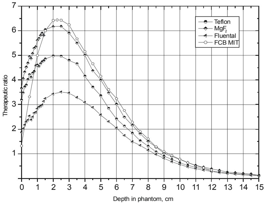
Fig. 11. Therapeutic ratio for different moderator materials as function of depth in phantom, moderator size 40x40x40 cm (proton energy 2.3 MeV) and reactor based beam [13].
