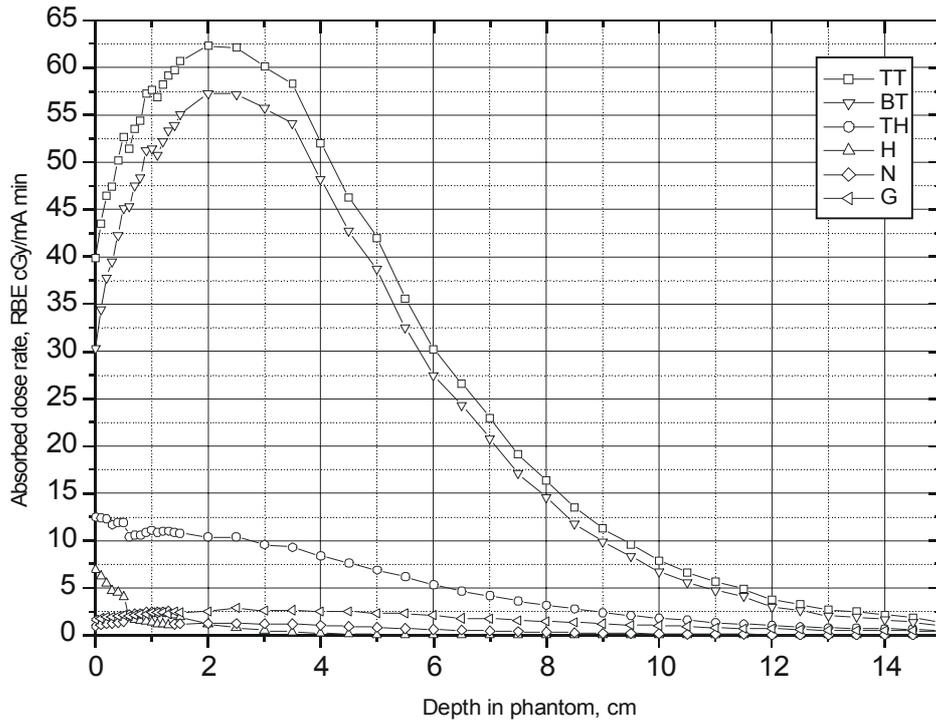
Fig. 9. Absorbed doses rates as function of depth in phantom. Polytetrafluoroethylene moderator, size 40x40x40 cm, proton energy 2.3 MeV, beam current 1 mA. TT – tumor total dose, BT – boron dose in tumor, HT – total dose in healthy tissue, H – proton recoil dose, N – dose from nuclear reaction with nitrogen, G – gamma ray dose.
