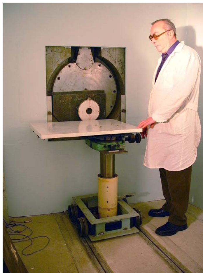
Fig. 7. The system to guide the neutron beam of the reactor into the irradiation room, and a movable platform to fix experimental animals.
