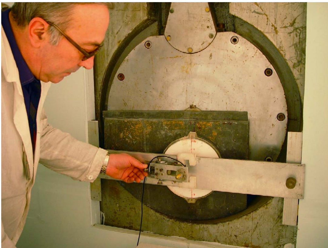
Fig. 10. Optical laser at the channel outlet.
