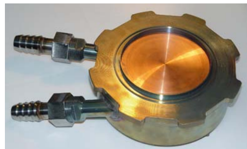
Fig. 10. Neutron producing target: 1 – backing with lithium layer, 2 – counter-plate with heater and container of lithium evaporation unit, 3 – silphon, 4 – water input, 5 – thermocouple, 6 – water output, 7 – bayonet.
