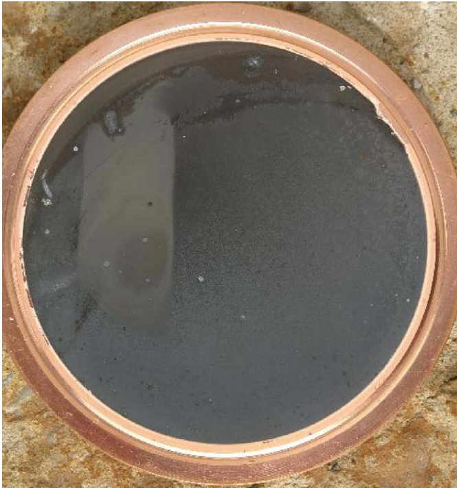
Fig. 5. Target substrate with lithium after neutron generation. The mark left by the beam can be seen on the left.
