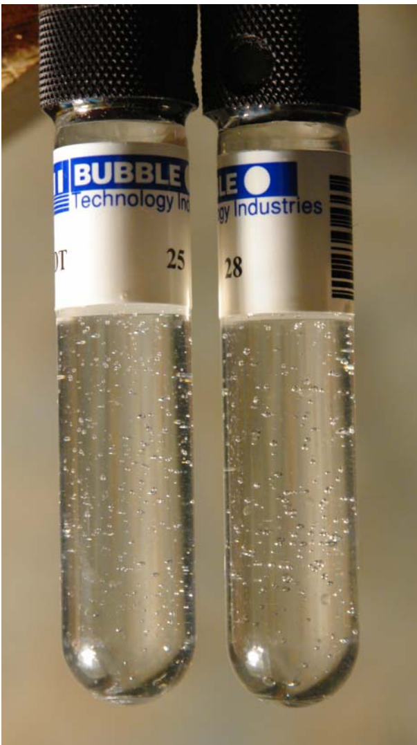
Fig. 7. The BDT detectors after neutron generation.
