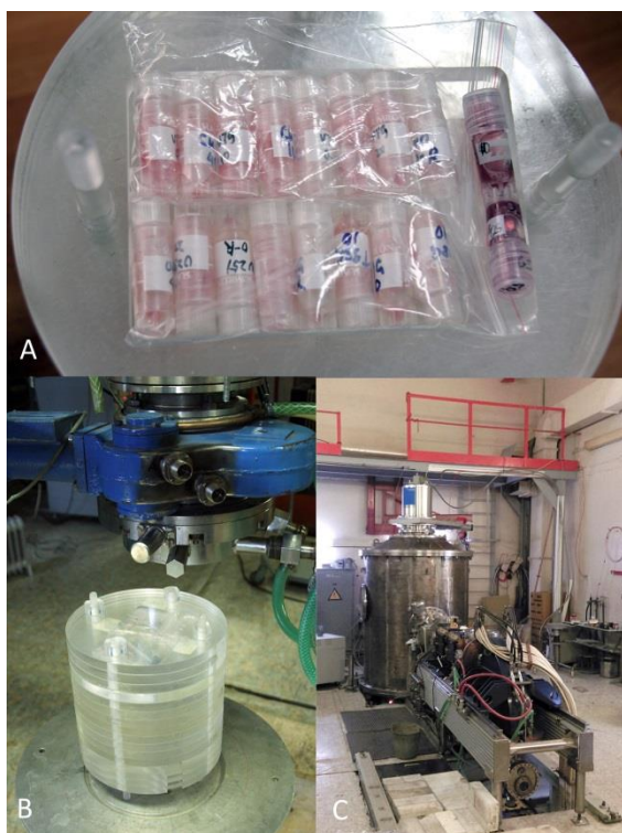
Fig.2 Irradiation experiments. U251MG cells placed in plastic vials (A) in a phantom made of organic glass under the lithium target (B) of the tandem accelerator with vacuum insulation (C) at the Budker Institute of Nuclear Physics, Novosibirsk Science City, Russian Federation..
