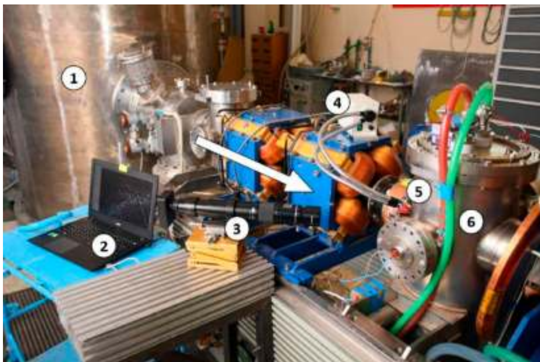
Figure 1. Experimental apparatus: ①, tandem accelerator with vacuum insulation; ②, computer; ③, remote microscope with a charge-coupled device camera; ④, booster-light; ⑤, fused quartz window; and ⑥, diagnostic vacuum chamber. The arrow schematically shows the direction of 2-MeV proton beam propagation.
