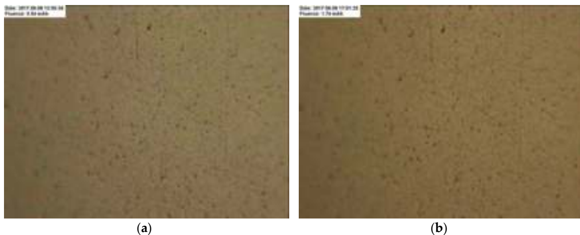
Figure 22. Images of the surface of Sample 5 during irradiation by a 2-MeV proton beam with varying integrals of the current: (a) 0.54, (b) 1.74 mA·h. The frame size is 9 mm horizontally and 4 mm vertically.
