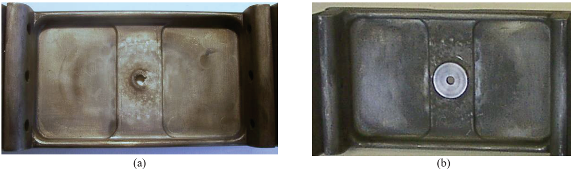
FIGURE 8. Extraction electrode modifications without and with the replaceable insert. (a) - deterioration of extraction electrode plate after 100 hours of operation; (b) - extraction electrode plate with the replaceable insert.
