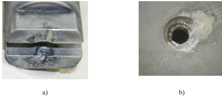
FIGURE 3. Discharge electrodes erosion. a) Cathode tips sputtering after 1000 hours of operation; b) erosion of emission aperture at anode cover after 3 month use.
