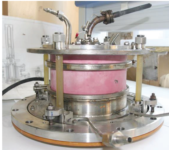
FIGURE 6. Source version with the replaceable IOS insulators.
