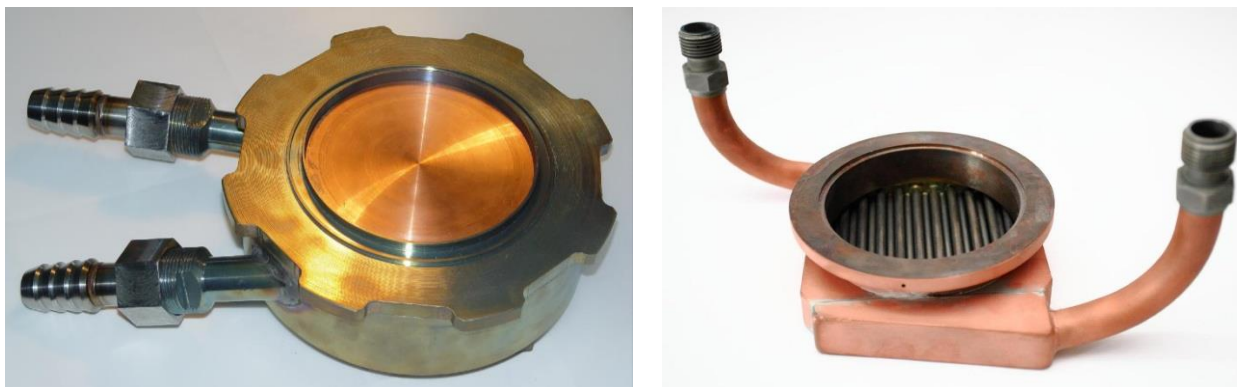
Fig. 3. Neutron producing target: target used in 2008-2018 (left), new target (right)
