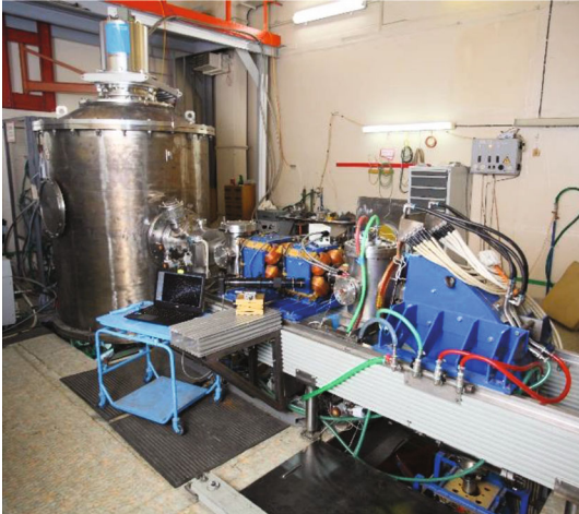
Fig. 2. Vacuum-insulated tandem accelerator: (left) photo, (right) schematic design: (1) H^- source, (2) magnetic lenses, (3) accelerator, (4) cryogenic pump, (5) intermediate electrodes, (6) high-voltage electrode, (7) gas stripping target, (8) bushing insulator, (9) high-voltage power supply, and (10) turbo-molecular pumps. The arrows show the direction of propagation of negative hydrogen ions ( H^- ) and protons ( p ).
