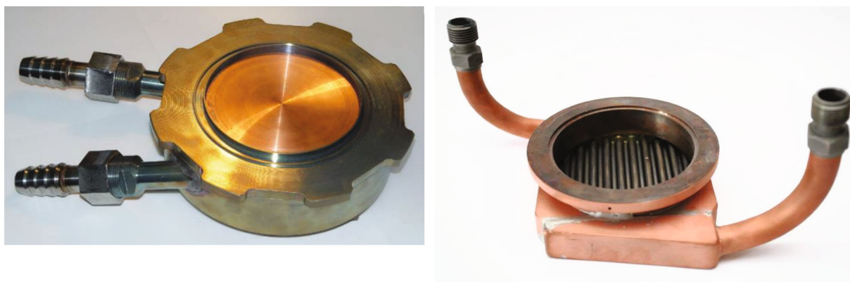
Fig. 3. Neutron-producing target: (left) the target used in 2008–2018 and (right) the new target.
