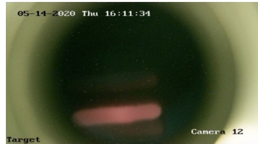
Figure 4: The argon beam glow and a beam of neutral atoms caused by the luminescence of the target lithium layer upon a twofold increase in the argon flow in the stripping target.
