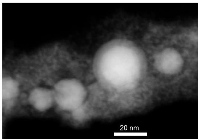
**Figure 3.** STEM view of NPs obtained by laser ablation of  $\text{Fe}_2\text{B}$  in isopropanol. Scale bar denotes 20 nm.
