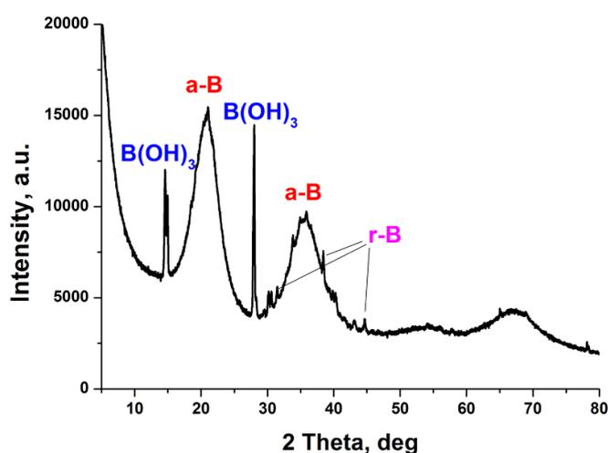
**Figure 4.** X-ray diffractogram of industrial boron powder. Label 'a-B' indicates amorphous B, 'r-B'—rhombohedral B.
