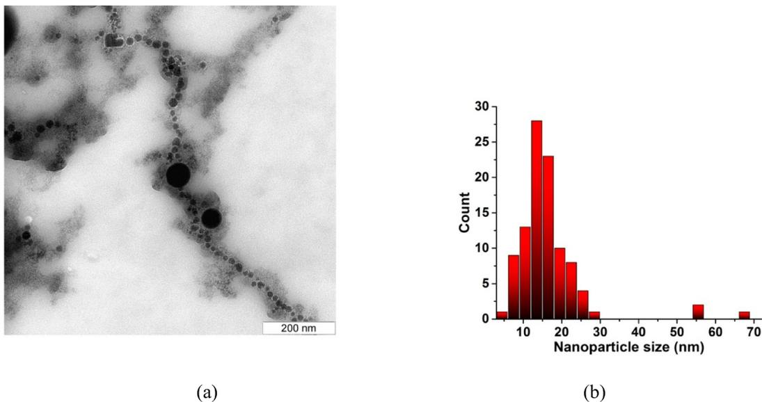
**Figure 2.** TEM view of NPs produced by laser ablation of  $\text{Fe}_2\text{B}$  target in isopropanol. Scale bar denotes 200 nm (a). Histogram of size distribution of NPs in figure 2 (b).
