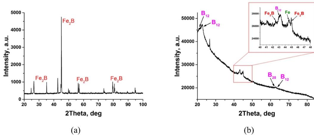
**Figure 1.** X-ray diffractograms of the initial  $\text{Fe}_2\text{B}$  target (a) and NPs generated by laser ablation of this target in liquid isopropanol (b).
