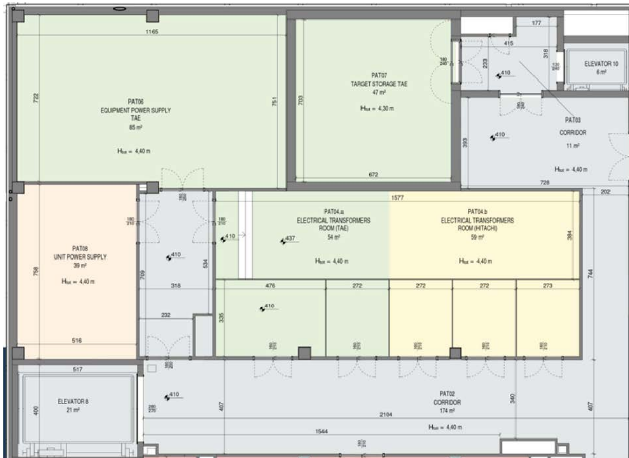
FIG. IV-5. The part of the first floor dedicated to BNCT (PAT07, PAT06, PAT04a).
