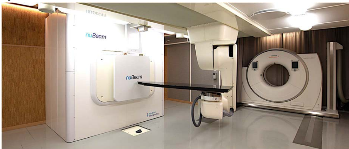
FIG. VI-1. The nuBeam treatment room at the Helsinki University Hospital cancer center illustrating the CT scanner (right), the robotic image-guided patient positioning system (middle), and the beam shaping assembly and the beam shutter (left).
