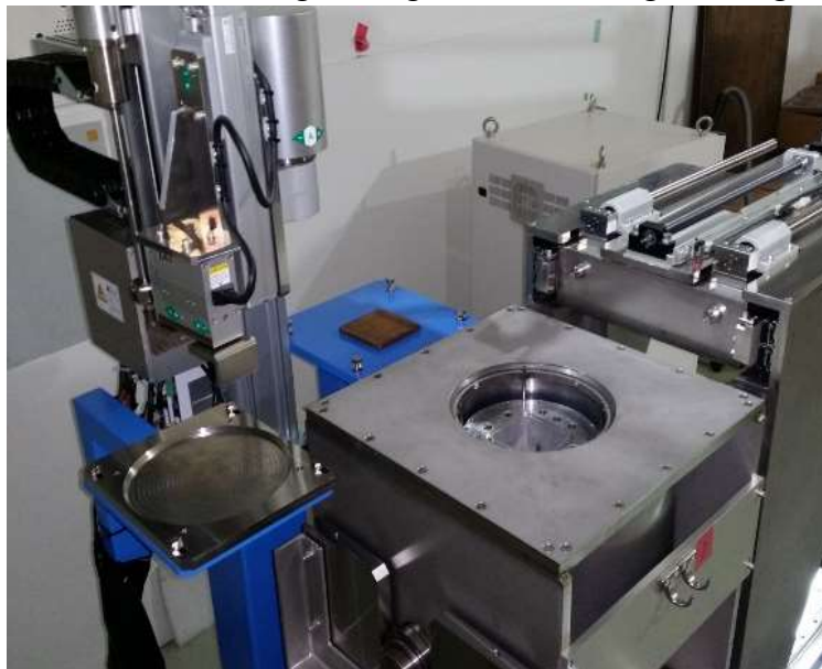
FIG. I-4. Remote target exchange device.
