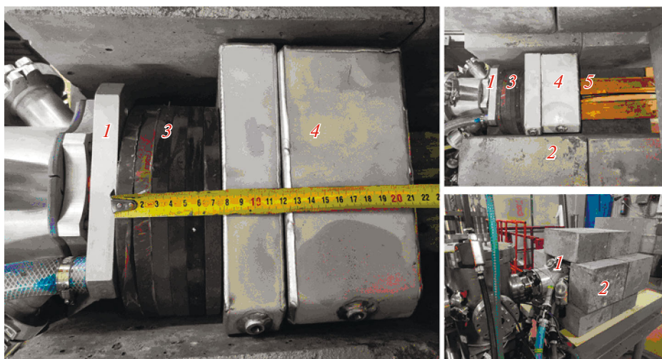
Fig. 3. Photos of the experiment: (1) lithium target, (2) concrete blocks enriched with boron, (3) plexiglass plates, (4) water/heavy water moderator, and (5) neutron detector.
