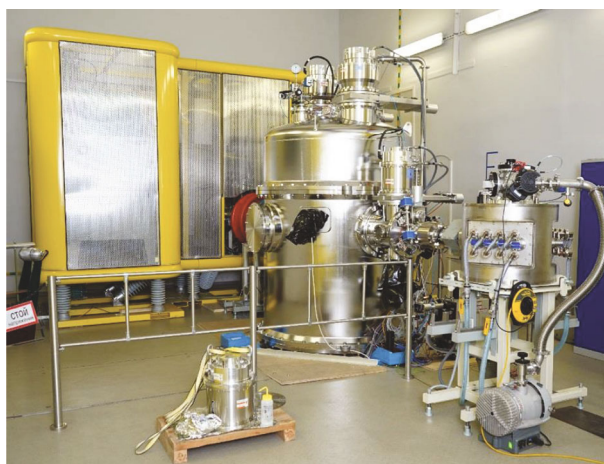
Fig. 2. Image of the VITA-II \alpha accelerator neutron source at the Institute of Nuclear Physics before transportation to China.
