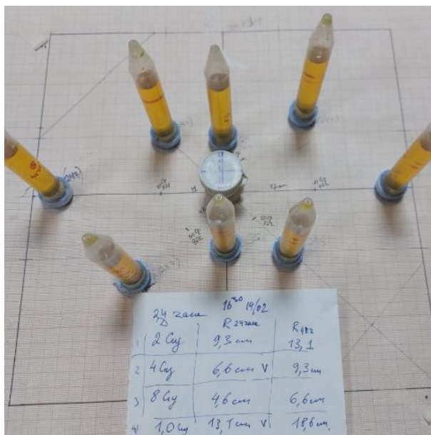
Fig. 3. Photo of dosimeter placement for calibration using a ^{137}\text{Cs} source
