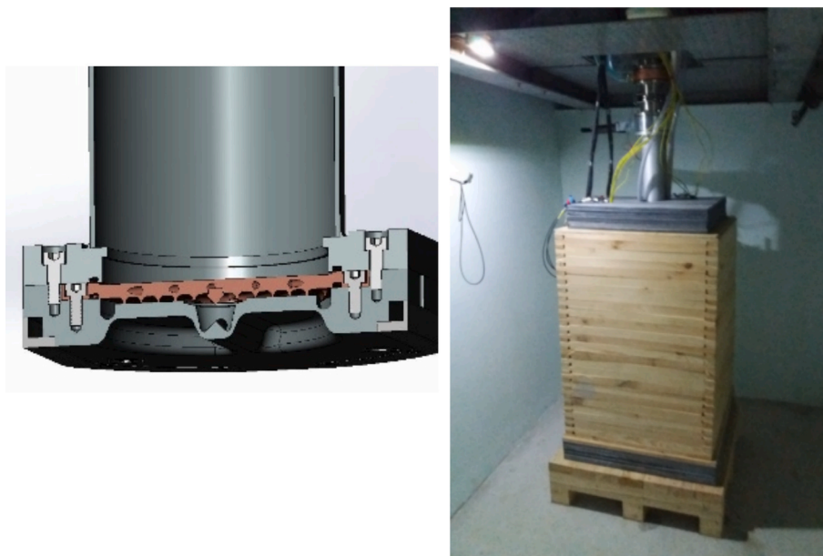
Fig. 3. Photos of the lithium target assembly (left) and concentrator (right).
