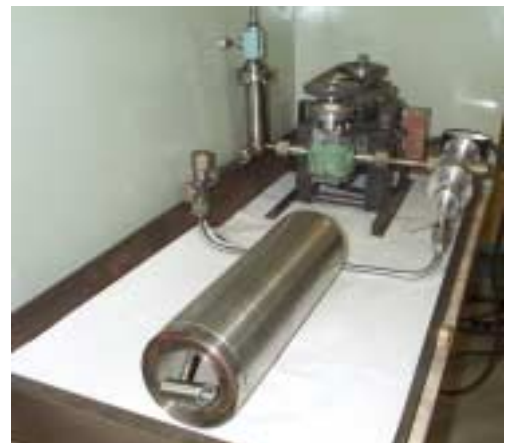
Fig. 6. Neutron production target before assembling (left) and liquid metal heat-carrier pump with heat-exchanger (right).
