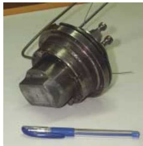
Fig. 2. Negative ion source with Penning geometry electrodes.
