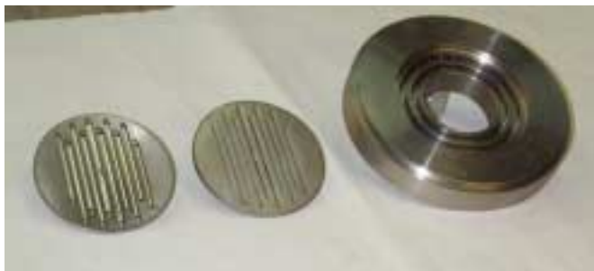
Fig. 6. Neutron production target before assembling (left) and liquid metal heat-carrier pump with heat-exchanger (right).
