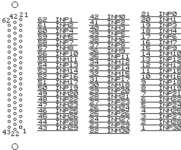
X1 connector provides 31 pair of ADC inputs. ADC inputs are not galvanically isolated each from other. They have common ground. A connection of ADC inputs with a signal source should be done by twisted pair.
