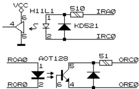
Output register design is based on transistor optocoupler and it is able to provide output current up to 32mA. Output voltage may be up to 30V.
