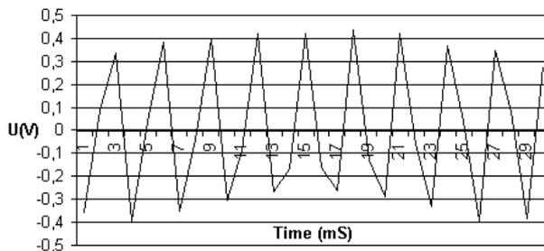
A fast measurements of low-frequency (300 Hz) signal. A data were collected in single channel mode, data rate was 1 kHz (time of measurements was 1 ms/point). A right picture presents a part of left picture (it is stretched in time).
