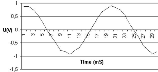
A fast measurements of low-frequency (50 Hz) signal. A data were collected in single channel mode, data rate was 1 kHz (time of measurements was 1 ms/point). A right picture presents a part of left picture (it is stretched in time).
